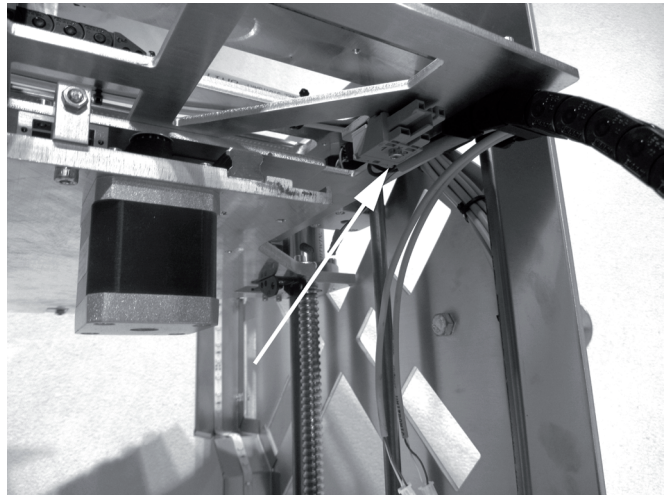
Install the plug connectors for the power supply of the heating plate with a cylinder head screw M3x16 at the bottom of the undertable.
